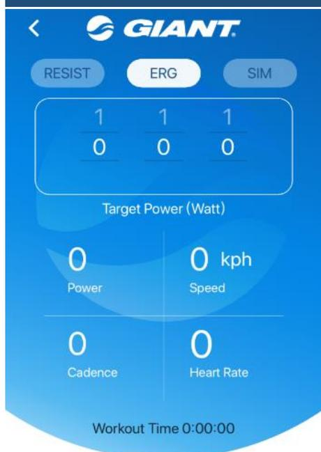
ERG mode: This is the training mode for constant power output. Enter the required power value. The CycloSmart will automatically generate the appropriate resistance according to the current speed to reach the chosen power value.
