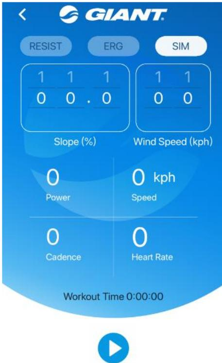
SIM mode: This is the training mode for simulation. Input slope (%) and wind speed (km/h) values, the CycloSmart will automatically generate appropriate resistance according on setting values and the current speed to reach a simulated real riding situation.
