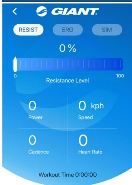
Resist mode: This is the training mode for constant resistance output. Adjust the required resistance output percentage. The resistance is constant output. It will not be changed by current speed.
